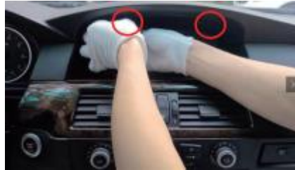
2. Remove the fixed screws from original monitor.
