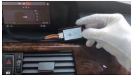
5. Connect AUX activator, start the car to enter the "Entertainment" menu, Then Check the activator indicator light: the light should be off.
