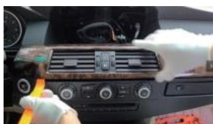
8. If you need add the AUX-in Port, Please follow below steps: Pry loose and take out the air conditioning decoration strip.
