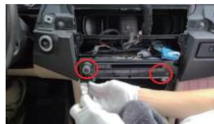
11. Remove the fixed screws from the Host.
