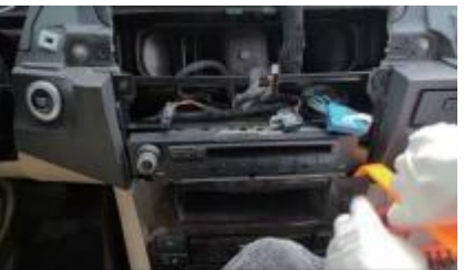
10. Pry and take out the panel of the storage box.
