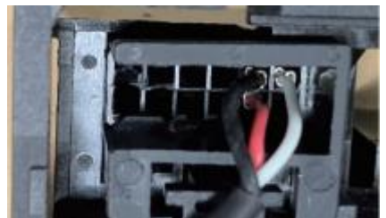
12. Take out the original harness. and plug three AUX wires into harness as picture show. After the installation is done, you can connect your phone into AUX Port to play music via AUX. (according to step 7)
