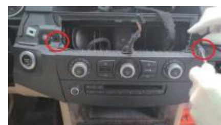
9. Remove the fixed screws of the panel.
