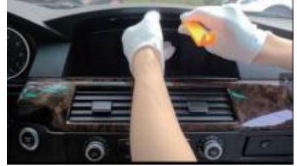
3. Pry loose and take out the original monitor.
