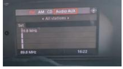
6. Long press the activator until the indicator light is on, check the "Entertainment" menu when "AUX" appears, release the key but keep the connection, wait 5 seconds, then turn off the engine and lock the car. Turn on the car again, if AUX Audio shows, then it has been activated and saved.
