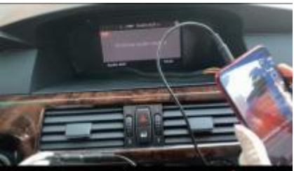
7. Connect phone with AUX IN to full test AUX function.
