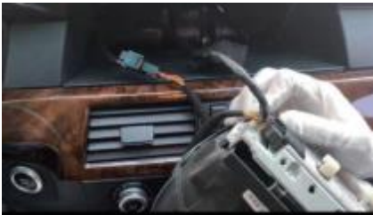
4. Connect well The AUX activator with original.
